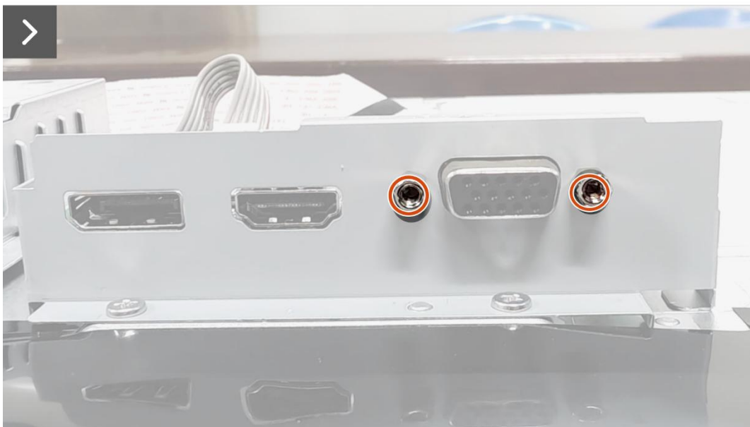
Figure 30. Removing the interface board
