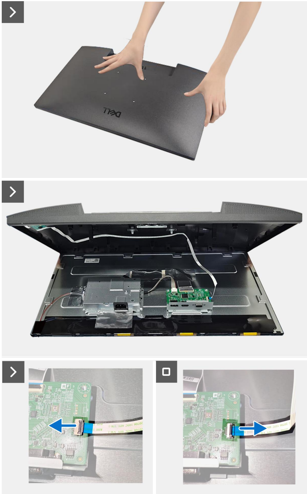
Figure 13. Removing the back cover
