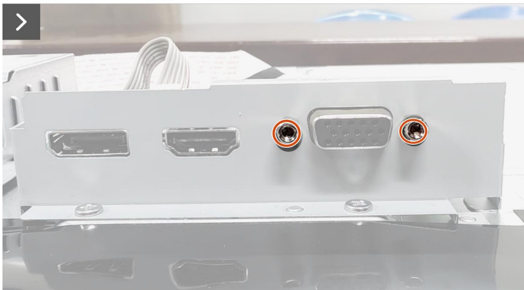
Figure 32. Installing the interface board
