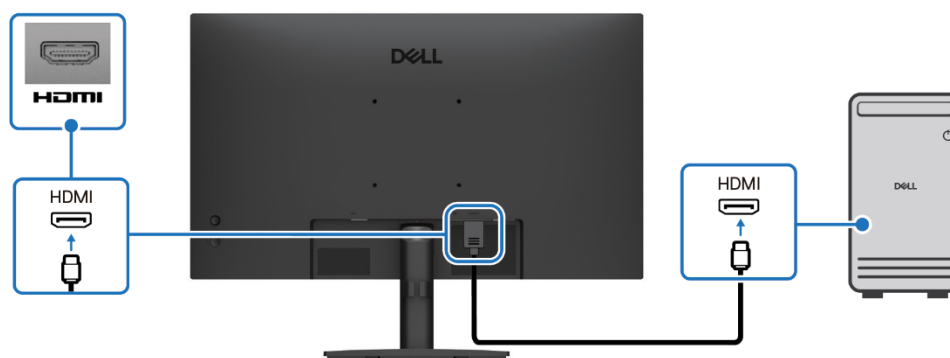
Figure 9. Connecting the HDMI cable
