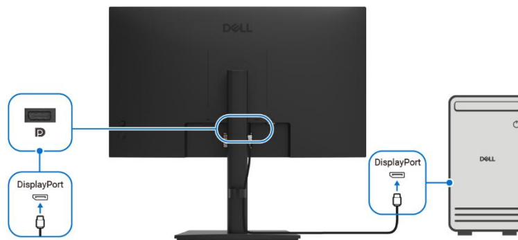
Figure 8. Connecting the DisplayPort cable
