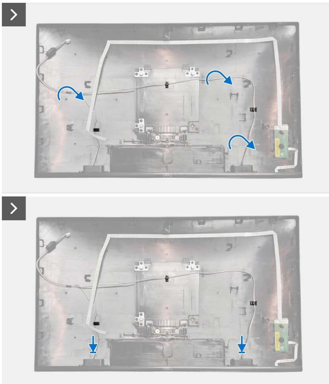
Figure 27. Installing the Speaker
