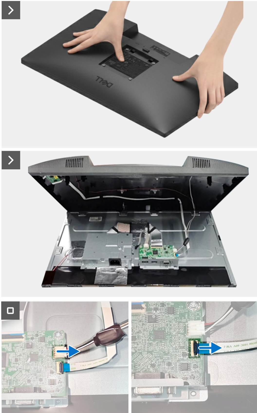
Figure 15. Removing the back cover
