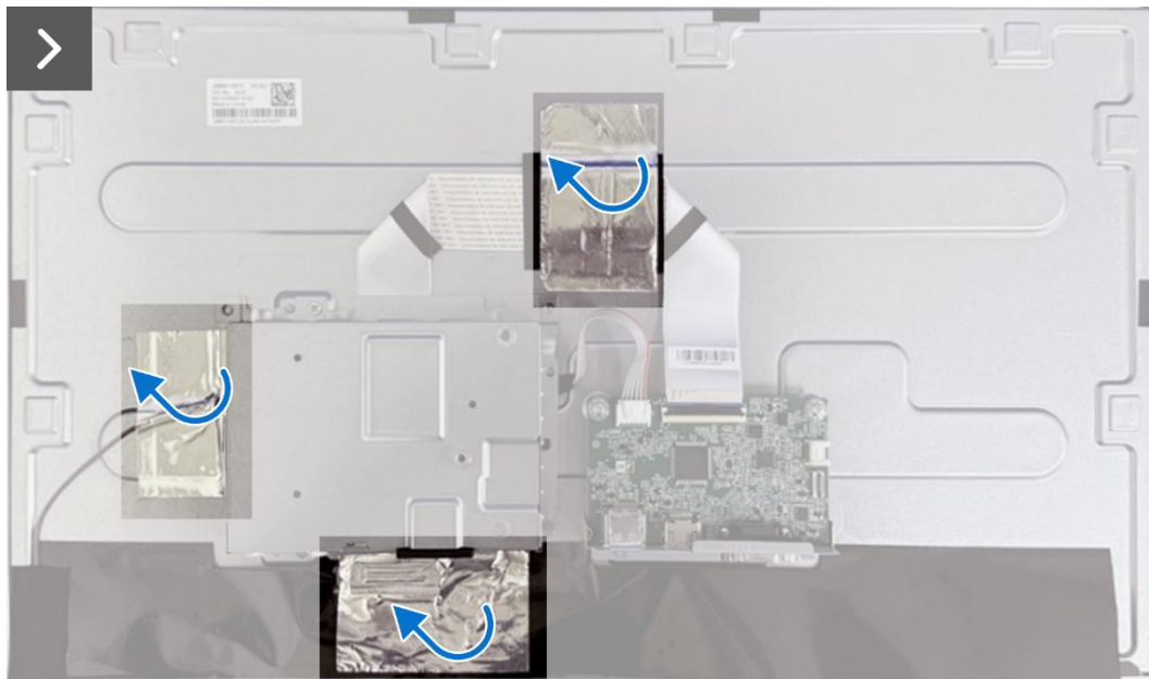
Figure 29. Removing the chassis assembly
