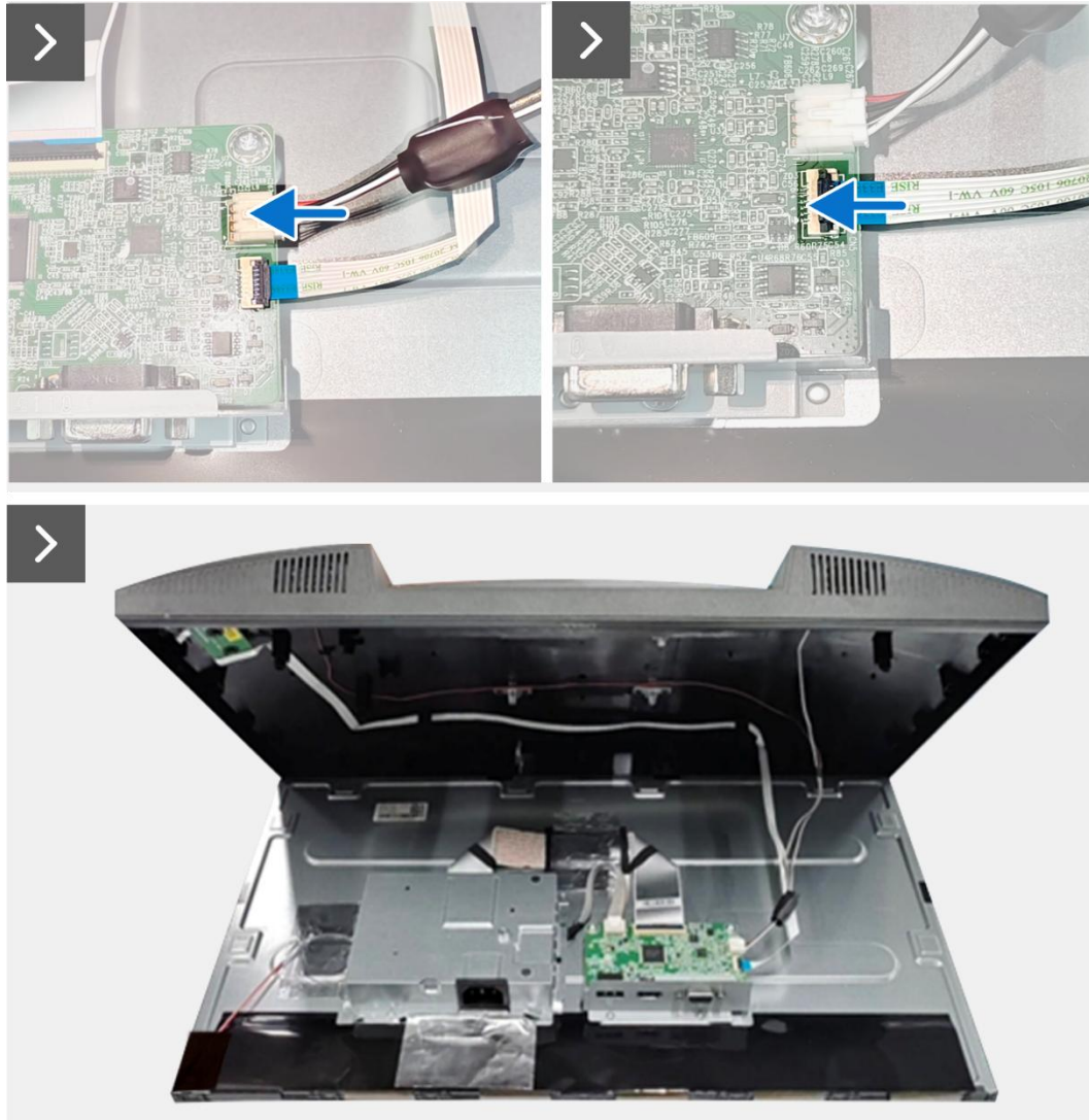
Figure 16. Installing the back cover
