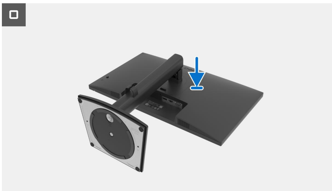
Figure 13. Installing the stand
