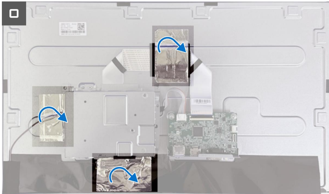
Figure 35. Installing the chassis assembly
