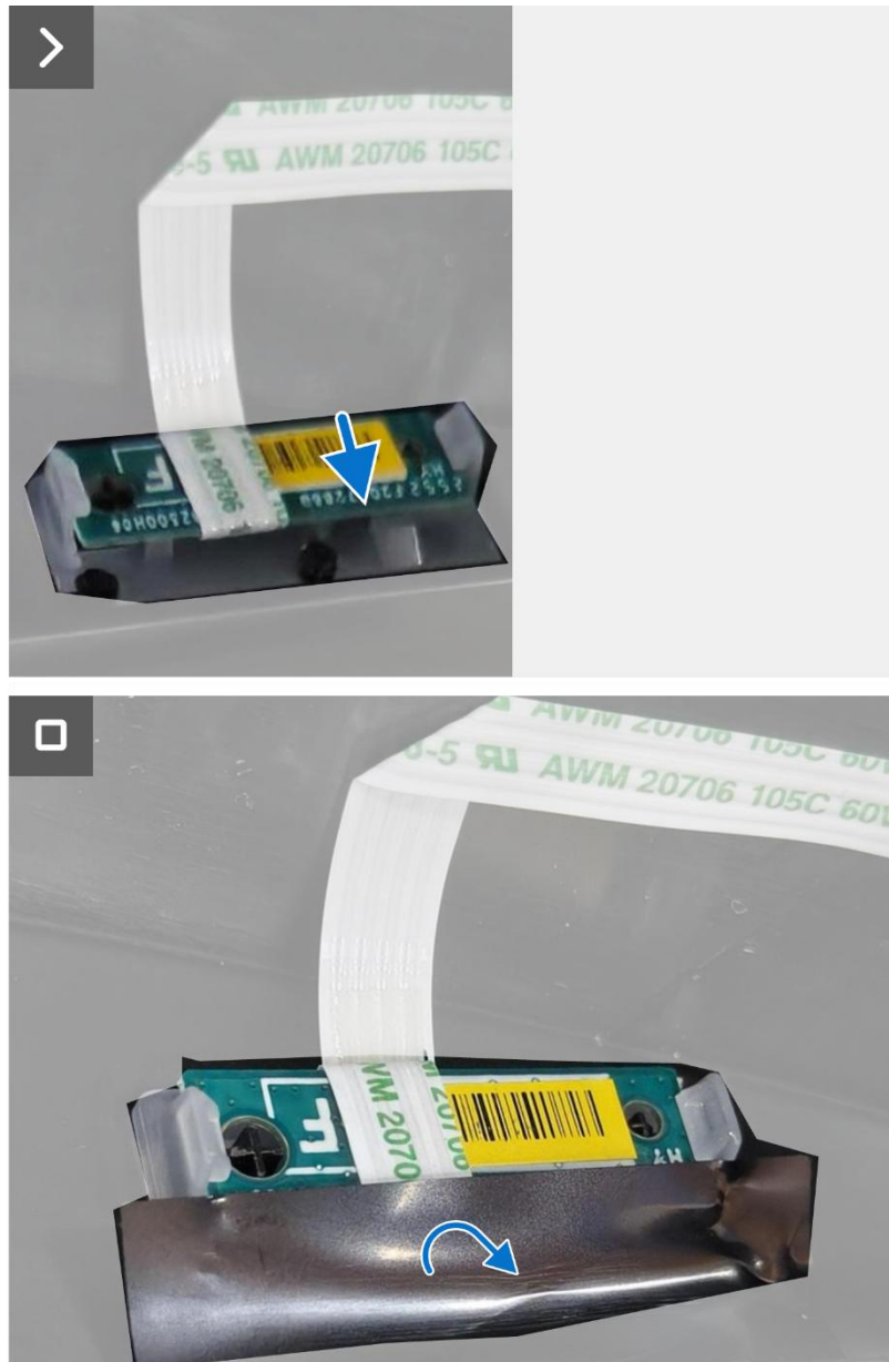
Figure 23. Installing the LED board
