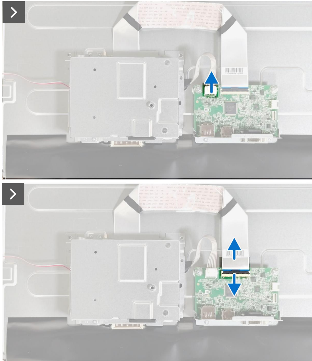
Figure 31. Removing the chassis assembly
