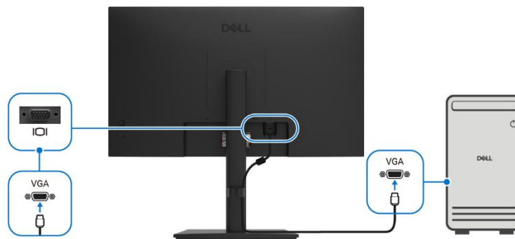
Figure 7. Connecting the VGA cable
