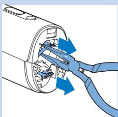
**6** Pull the battery connectors off the battery terminals with long nose pliers.
