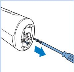
**3** Insert an awl or another pointed tool into the bottom cap of the appliance and pry off the bottom cap.
