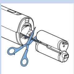
**8** Cut the two wires one at a time to ensure that no mishaps due to possible residual charge occur.
