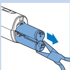
**7** Pull the rechargeable batteries out of the appliance with long nose pliers.
