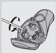
**3** Undo the two screws in the hair chamber.
