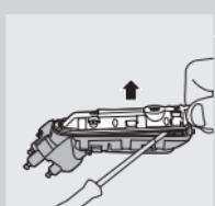
**8** Remove the power unit cover with a screwdriver.
