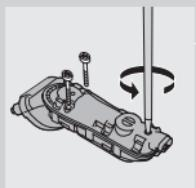
**7** Undo the three screws in the power unit.
