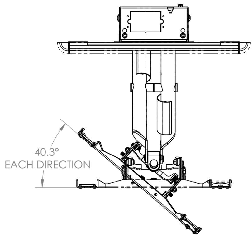
NOTE: CUSTOM INTERAFCE BRACKET NOT SHOWN. THE CUSTOM INTERFACE BRACKET NEEDED FOR YOUR DISPLAY WILL ADD BETWEEN 1/2" AND 2" IN DEPTH AND MAY AFFECT LOCATION OF DISPLAY ON THE MOUNT. SEE MSB-XXXX DRAWING ALSO.
