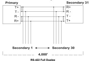
Note: When the distance between both ends of the installation is large and/or the transmitted signals are unstable, insert  $120\Omega$  terminal resistors between pins 1 and 2 and between pins 3 and 4 on the terminal blocks of the two units at each end of the installation.
