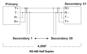
Note: When the distance between both ends of the installation is large and/or the transmitted signals aren't stable, insert a  $120\Omega$  terminal resistor between pins 1 and 2 on the terminal blocks of the two units at each end of the installation.
