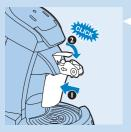
6 Slide the milk container unit into the coffee machine (1) and push down the milk container lever ('click') (2).
