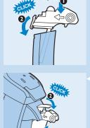
5 Slide the milk container unit into the coffee machine (1) and push down the milk container lever ('click') (2).
