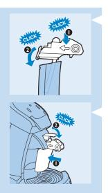
6 To fasten the milk container lid onto the milk container, first push the front of the milk container lid onto the edge of the milk container ('click') (1) and then push the rear end onto the milk container ('click') (2).
