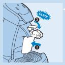
3 Slide the milk container unit into the coffee machine (1) and push down the milk container lever ('click') (2).
