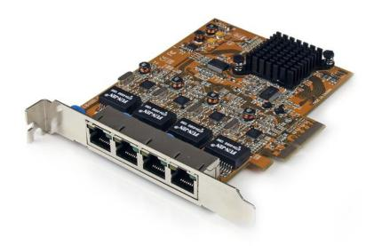
The ST1000SPEX42 4-port Ethernet Card is an IEEE 802.3/u/ab standards compliant PCIe network adapter, which adds connections to up to four separate high-speed Gigabit networks from a single desktop client, server or workstation.
