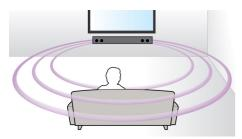
Philips Virtual Surround Sound produces rich and immersive surround sound from a less than five-speaker system. Highly advanced spatial algorithms faithfully replicate the sonic characteristics that occur in an ideal 5.1channel environment. Any high quality stereo source is transformed into true-to-life, multichannel surround sound. No need to purchase extra speakers, wires or speaker stands to appreciate room-filling sound.
