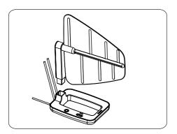
2 Connect the other end of the built-in coaxial cable to the input on the TV receiver.
