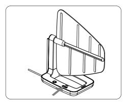
3 Tilt or swivel the UHF log periodic antenna towards the transmitter until the reception is achieved.
