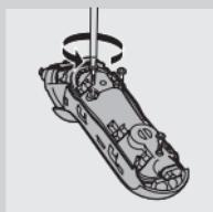
**5** Undo the three screws in the sealed power unit.
