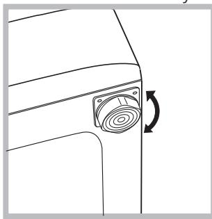
Levelling the machine correctly will provide it with stability, help to avoid vibrations and excessive noise and prevent it from shifting while it is operating. If it is placed on carpet or a rug, adjust the feet in such a way as to allow a sufficient ventilation space underneath the washing machine.
