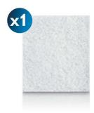
The kit contains 1 x triple-layer motor filter. This filter prevents fine dust from reaching the motor and damaging it. The filter should be replaced once a year.
