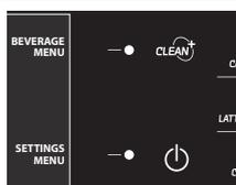
Flashing red light. Machine in Stand-by.
