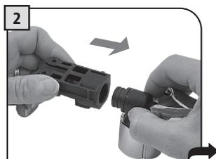
2 Insert the outer fitting in the inner fitting. Refer to the arrow in the figure for the direction of insertion.
