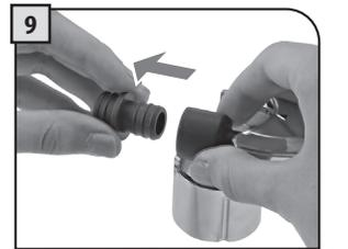
9 Remove the internal fitting.
