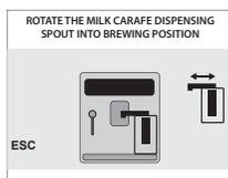
A beverage with milk has been selected. The machine requires the carafe handle spout to be placed into dispensing position.
