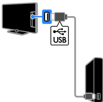
1. Connect the USB hard drive directly to the TV, or if you intend to connect other USB devices in future, connect the USB hard drive through a USB hub.
