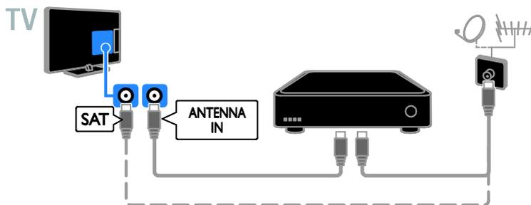
Connect the satellite or digital TV receiver to the TV with an HDMI cable.
