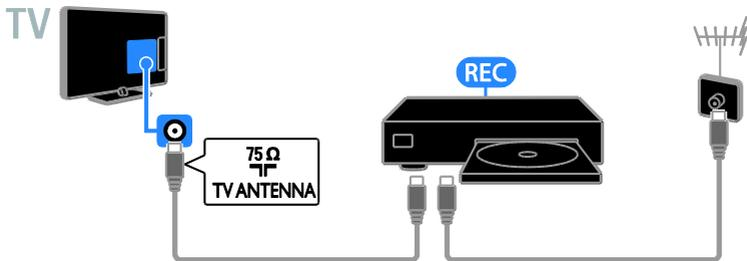
Connect the recorder to the TV with an HDMI cable.
