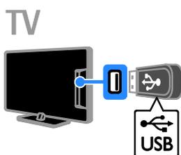
Connect the USB flash drive with a USB cable to the TV.
