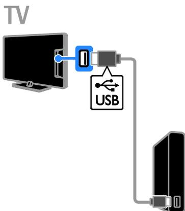
Connect the USB hard drive to the TV with a USB cable.
