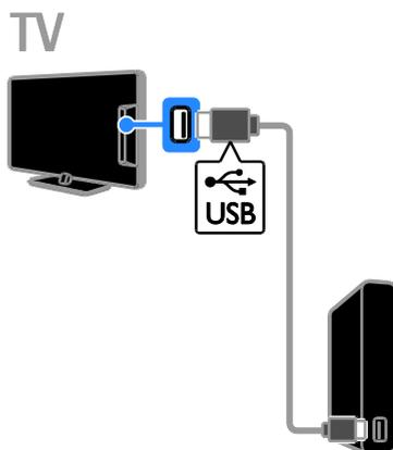
1. Connect the USB hard drive directly to the TV, or if you intend to connect other USB devices in future, connect the USB hard drive through a USB hub.
