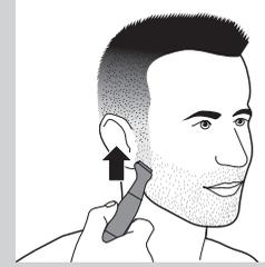
*Note: You can use the precision trimming head with the trimmer teeth pointing towards the skin. You can also use it with the flat part touching the skin and the teeth pointing in the direction in which you move the appliance.*
