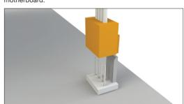
Position the cooler over the CPU.
