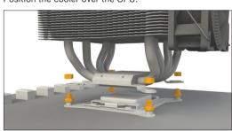
Place the hexagonal nuts (8) over the spacer nuts (7) and progressively tighten these in a crosswise manner until firm
