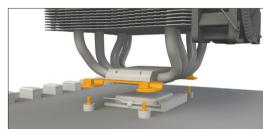
(10) and affix by turning the AMD M3x15 screws (10) from the rear side of the motherboard.
