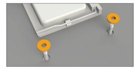
Now fasten the backplate on the front side of the motherboard using the C-profile spacers (12) by pressing these onto the notches in the AMD M3x15 screws (10) until they click in.
