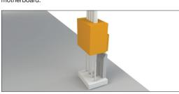
Position the cooler above the CPU, passing the attached  $\ensuremath{\mathsf{AMD}}$ mounting brackets (5) over the projecting AMD M3x15 screws
