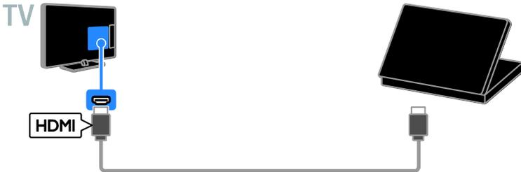
(For certain sets only.) Connect the computer with a DVI-HDMI cable and an audio cable to the TV.
