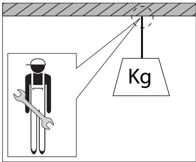
**EN:** Always consult a professional in advance, for choosing the right fastener for a secure mounting of the product. Take into account the weight of the product and the material of the mounting surface.
