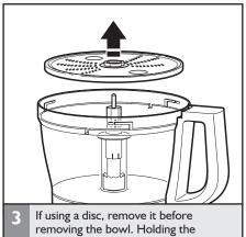
3 If using a disc, remove it before removing the bowl. Holding the disc by the 2 finger grips, lift it straight up. Remove the adapter.
