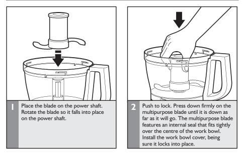
**IMPORTANT:** The multipurpose blade and dough blade\* can only be used with the work bowl.
