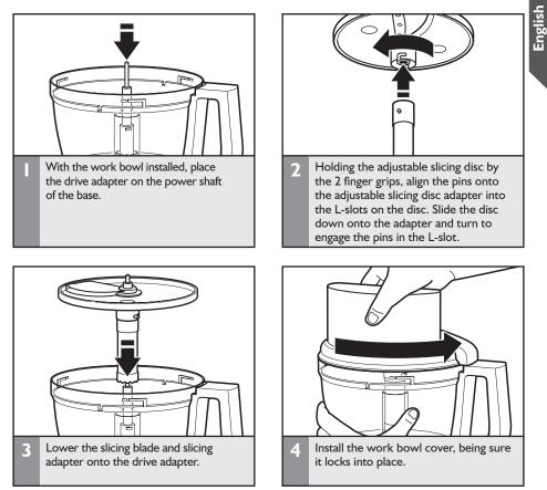
TIP: You may need to turn the disc/drive adapter until it drops down into place.
