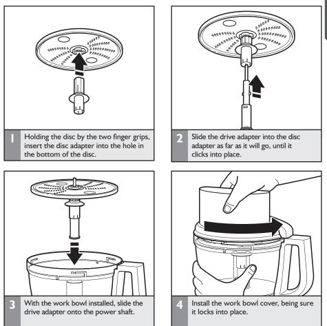
**TIP:** You may need to turn the disc/drive adapter until it drops down into place.
