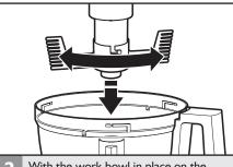
2 With the work bowl in place on the base, place the egg whip on the power shaft. Rotate the egg whip so it falls into place on the power shaft.
