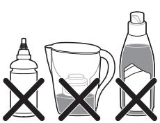
**Caution: Do not use perfumed water, water from a tumble dryer, rainwater, vinegar, mineral water, magnetically treated water (Aqua+), water from a drinking water filter, starch, descaling agents, ironing aids, salt or chemicals in the water tank. These types of water have been tested. They are not suitable and may even cause damage to the appliance. If you use any of these types of water, your guarantee becomes invalid.**
