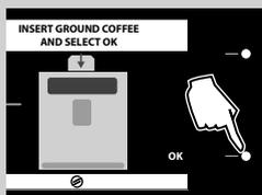
4 Press the “OK” button. The machine starts dispensing water.
