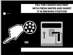
**11** Empty the milk carafe and fill it with fresh water. Insert it back in the machine. Press the “OK” button.
