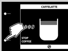
8 Once the milk has been poured, the machine brews coffee. The brewing can be stopped earlier by pressing the “**STOP COFFEE**” button.
