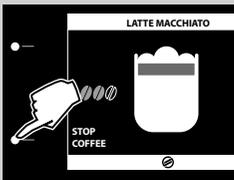
8 Once the milk froth has been poured, the machine brews coffee. The brewing can be stopped earlier by pressing the “**STOP COFFEE**” button.
