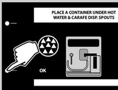
**12** Empty the container and place it back under the hot water/steam wand and milk dispensing spout of the carafe. Press the “OK” button.
