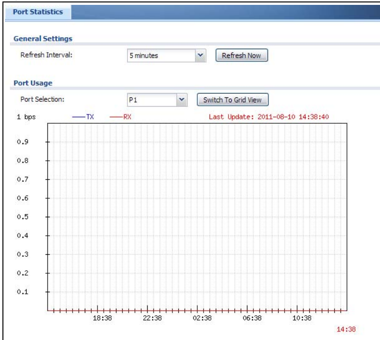
Figure 95 Monitor > System Status > Port Statistics > Switch to Graphic View
