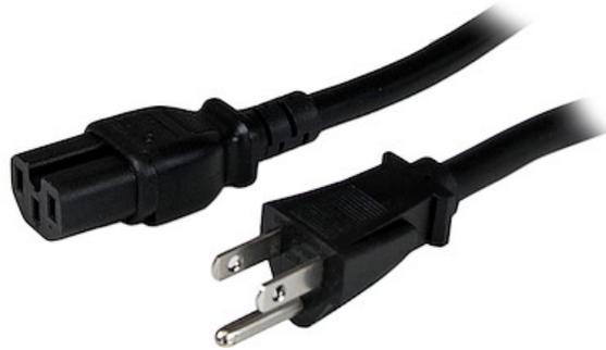
The PXT515C154 4-foot Computer Power Cord features a C15 connector rated for high-temperature equipment, as well as 14 AWG wire suitable for high power connections - a reliable solution for connecting to NEMA 5-15P Power Distribution Units (PDU) located in switchgear rooms and data center environments, or large server applications that require a higher rated, heavier gauge cable.
