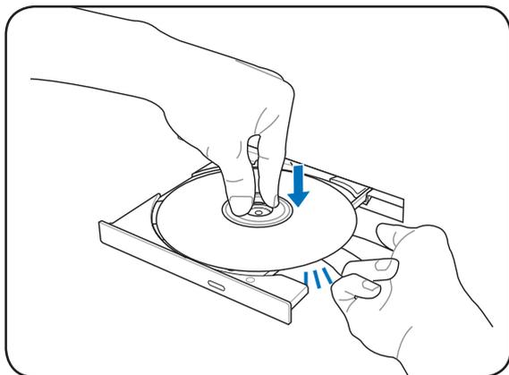
4. Slowly push the drive's tray back in. The drive will begin reading the table of contents (TOC) on the disc. When the drive stops, the disc is ready to be used.
