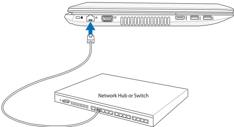
Network cable with RJ-45 connectors
