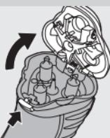
**1** Switch off the shaver, remove the powerplug from the wall socket and pull the appliance plug out of the shaver.
