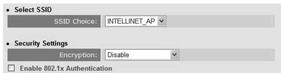
The screenshot shows a configuration interface for a wireless access point. It has two main sections: "Select SSID" and "Security Settings". In the "Select SSID" section, the SSID choice is set to "INTELLINET\_AP". In the "Security Settings" section, the encryption is set to "Disable" and the "Enable 802.1x Authentication" checkbox is unchecked.
