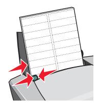
**Note:** If you are using letter size sheets of labels, adjusting the paper guide may not be necessary.
