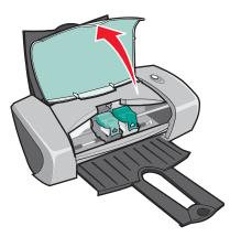
The cartridge carrier moves to the loading position, unless the printer is busy.
