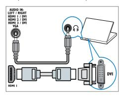
HDMI cable and HDMI-DVI adaptor (side HDMI and AUDIO IN L/R)
