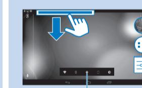
Power control widget: On/ off switches for Wi-Fi, Bluetooth, GPS, background sync (for some apps, like mail) and screen brightness
