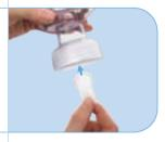
Wash your hands thoroughly. Click the white valve into the pump body so that it fits securely into the small round hole. Make sure the pointed side of the valve is facing down.
