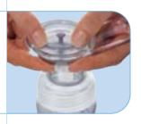
Fit the silicone diaphragm into the pump body. Ensure a perfect seal around the rim by pressing down with your fingers. (This is easier if assembled while the diaphragm is wet.)
