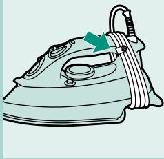
**1** Remove the mains plug from the wall socket and set the steam control to position O.
