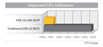
Test results were obtained using an Intel® Ivy Bridge system, StarTech.com add-on USB 3.0 cards, a UASP-enabled StarTech.com enclosure, and a SATA III solid state drive.
