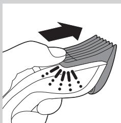
Use the trimmer without the trimming comb to clip hair close to the skin (0.5mm) or to contour the neckline and sideburns.
