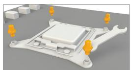
Installation of the mounting brackets
