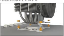
Place the hexagonal nuts (8) over the spacer nuts (7) and progressively tighten these in a crosswise manner until firm using the hexagonal wrench (13).
