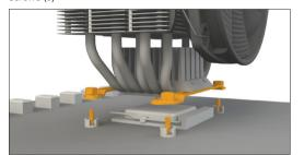
and affix by turning the M3x16 screws (9) from the rear side of
