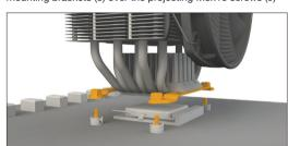
and affix by turning the M3x16 screws (9) from the rear side of the motherboard.
