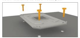
On the front side of the motherboard, pass the AMD washers (12) over the projecting M3x16 screws (9) to cover the motherboard screw holes.
