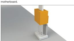
Position the cooler over the CPU.
