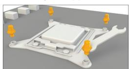
Installation of the mounting brackets
