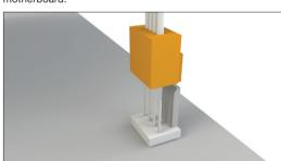
Position the cooler over the CPU.
