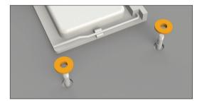
Now fasten the backplate on the front side of the motherboard using the C-profile spacers (11) by pressing these onto the notches in the M3x16 screws (9) until they click in.
