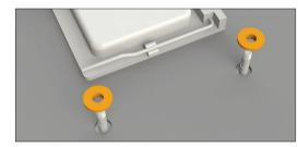
Now fasten the backplate using the C-profile spacers (11) by pressing these onto the notches in the M3x16 screws (9) until they click in.
