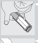
9 Pry the 2 AA-sized cylindrical nickel-cadmium batteries loose by inserting the screwdriver on the sides of the two batteries in the locations shown in the figure.
