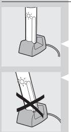
Sonicare comes with the batteries completely discharged and should be charged for at least 24 hours during the first few days of use. It is recommended that you keep your Sonicare in the charger when not in use to maintain a full battery charge. It takes at least 24 hours to fully charge the battery of your Sonicare toothbrush.
