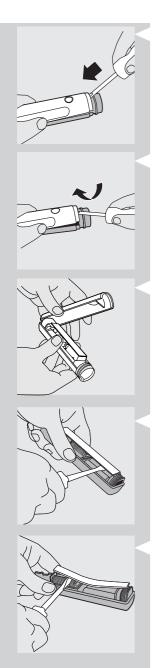
4 Now, insert the screwdriver into the middle slot located on the top front part of the handle as shown and push the blade in as far as it will go.
