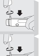
3 Remove the screwdriver and repeat the above instruction using the other slot located on the opposite side of the handle. Twist the blade and the housing will continue to split.
