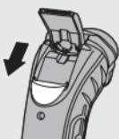
**1** Open the trimmer by pushing the slide downwards.
