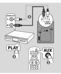
Use the red/white audio cables to connect the system's AUX/CDR IN (R/L) terminals to the AUDIO OUT terminals on the other audio/visual device (such as a TV,VCR, Laser Disc player, DVD player or CD recorder)
