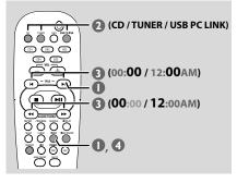
Press and hold **TIMER** on the remote until icon starts flashing. OR
