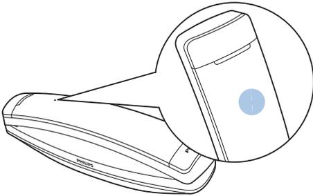
Charge your handset by docking it in either direction. When the handset is placed correctly on the base station, you hear a docking tone (see 'Set the docking tone' on page 31). The LED at the back of the handset flashes once.
