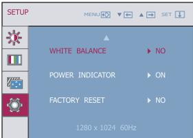
**WHITE BALANCE** If the output of the video card is different from the required specifications, the color level may deteriorate due to video signal distortion. Using this function, the signal level is adjusted to fit into the standard output level of the video card in order to provide the optimal image. Activate this function when white and black colors are present in the screen.
