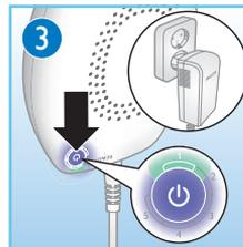
**EN** Plug in the appliance and switch it on. The light of intensity 1 goes on and the fan inside starts.
