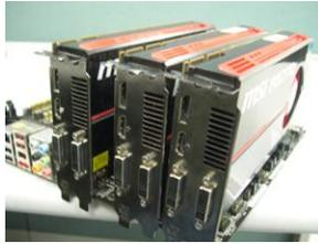
Step 2. Use one CrossFire™ Bridge to connect Radeon graphics cards on PCIE2 and PCIE4 slots, and use the other CrossFire™ Bridge to connect Radeon graphics cards on PCIE4 and PCIE5 slots. (CrossFire™ Bridge is provided with the graphics card you purchase, not bundled with this motherboard. Please refer to your graphics card vendor for details.)
