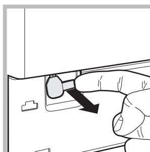
3. remove the cover panel on the lower front part of the washing machine (see overleaf).
