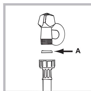
2. Insert seal A into the end of the inlet hose and screw the latter onto a cold water tap with a 3/4 gas threaded mouth (see figure). Before making the connection, allow the water to run freely until it is perfectly clear.
