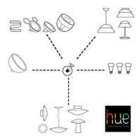
You can connect up to 50 bulbs or lamps to your existing Philips hue bridge. Simply begin with any of the available extension kits and start adding Philips hue bulbs or Philips Friends of hue products in any combination. With a tap of your finger, you can now control any connected lighting in your home.
