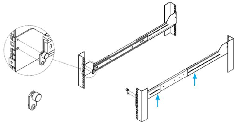
3. Slide the shelf assembly onto the rails.
