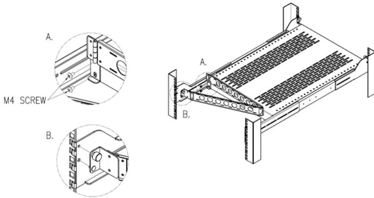
**Note:** The Cable Management assembly can be attached to either side of the shelf.
