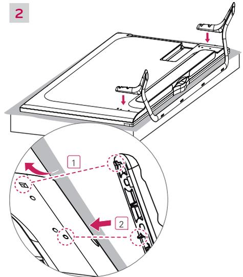
**1** Attach the stand to the TV using the upper mounting hole on the back of the TV.
