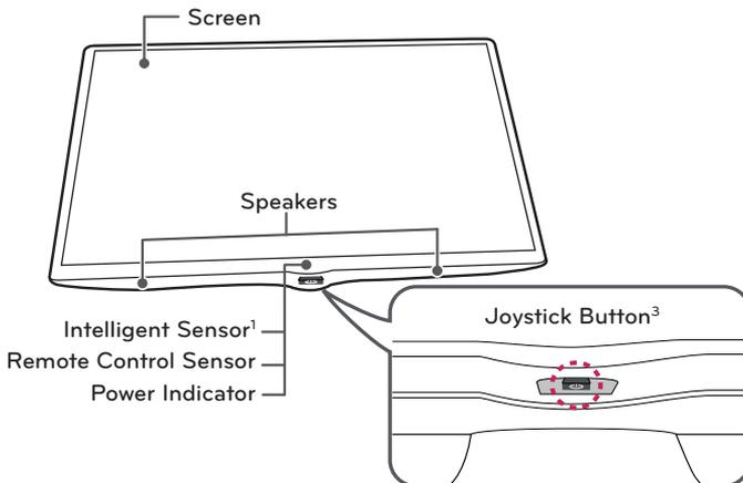
1. Intelligent sensor - Adjusts the image quality and brightness based on the surrounding environment.
