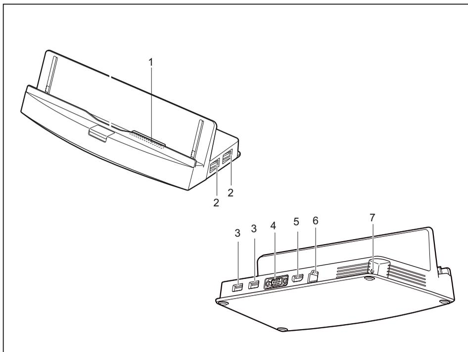
1 = Connector on the cradle for the docking port of the Tablet PC
