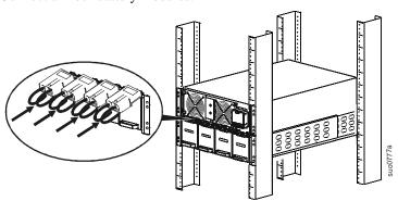
• Reinstall the battery compartment doors.
