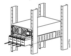
**6** After the UPS is hardwired to branch circuit mains complete steps 6-8. Connect all four battery modules.
